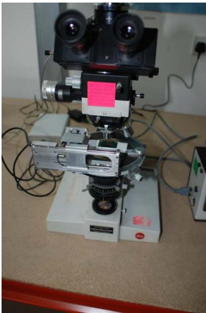
The stepper can also be fitted to older microscope stages, and even the smaller stages fitted to earlier models
