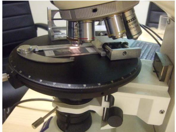
**Stepper assembly** and attached communications leads. Attaches to all major POL microscopes in use for geology. The stepper has a low profile on the stage, with a high-rise part well away from the microscope's objectives and turret.
